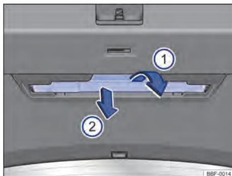
Fig. 49 Na tampa traseira: suporte para o triângulo de segurança.
