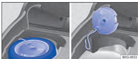
Fig. 186 Remover o subwoofer.
