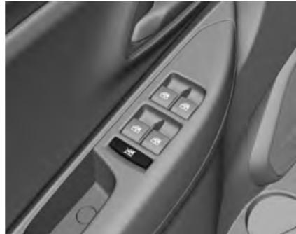
Pressione o interruptor
