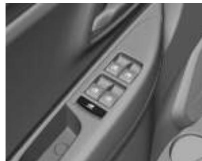
Pressione o interruptor
