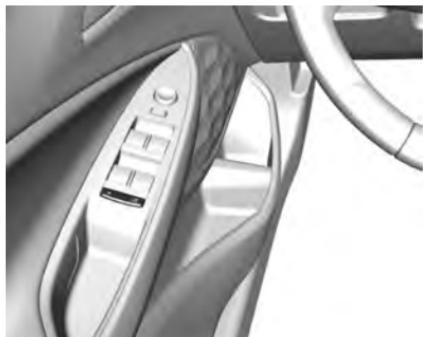
Pressione o interruptor
