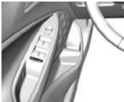
Pressione o interruptor
