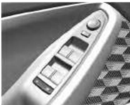
Pressione o interruptor
